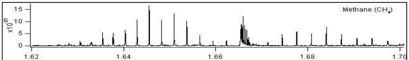
Infrared Absorption spectra of Methane (Absorbance vs. Wavelength (µm))
