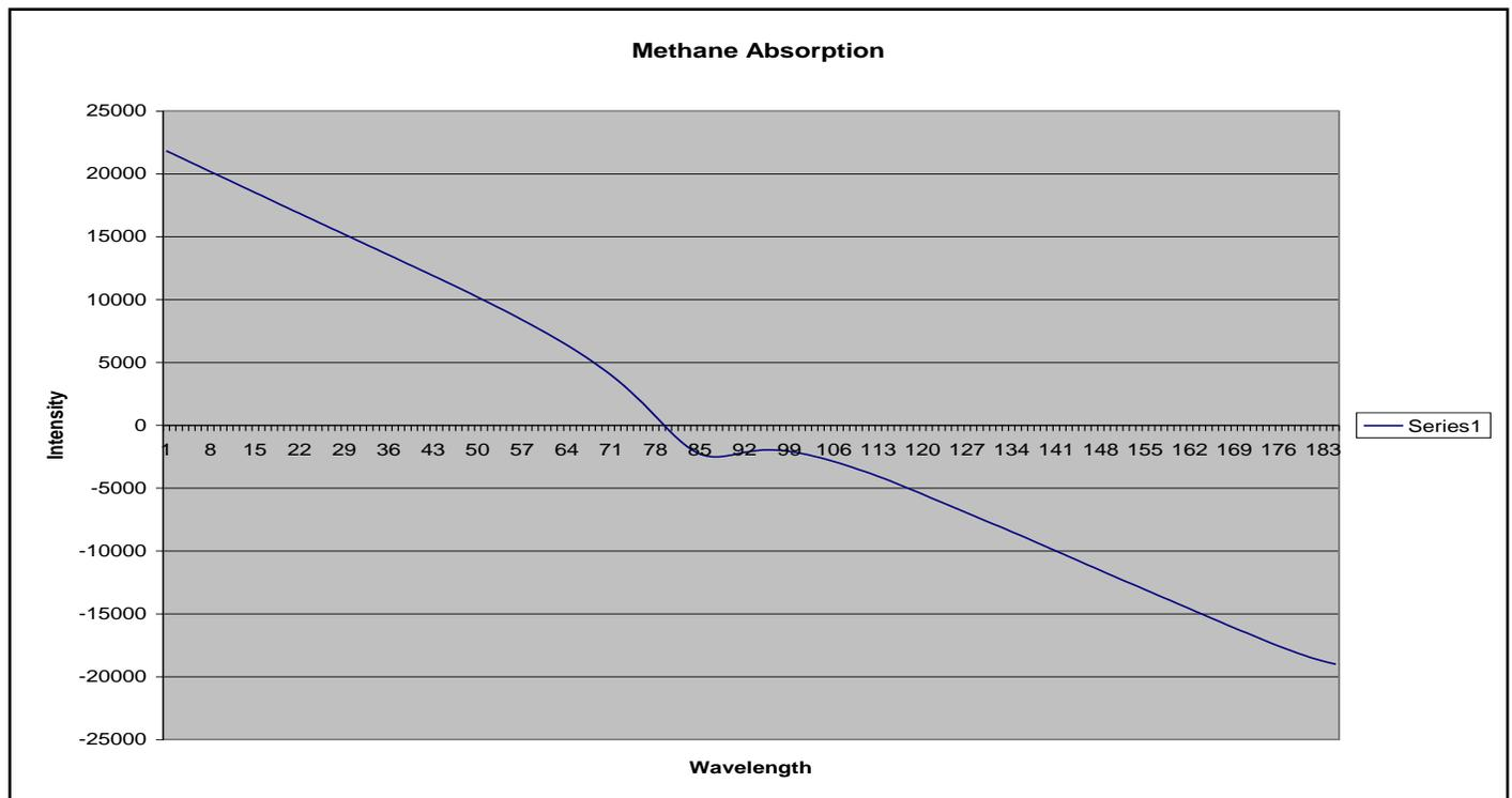
Laser intensity scan over 100ppm-m Methane @1.645µm absorption feature
